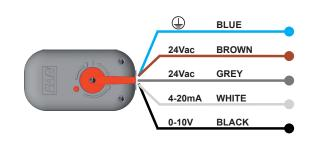
To control the opening and closing of the zone valve through the actuator, simply connect the blue cable to neutral, the brown cable to phase and the black cable to the 0-10V control unit (or the white cable if the regulation is 4-20mA). The grey cable is used to invert the starting point of the actuator and, as far as our applications are concerned, we suggest to leave it always under power.
