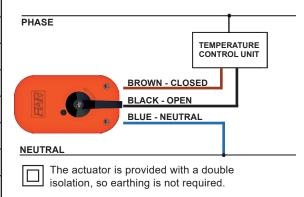
To control opening and closing of a zone valve via an actuator, connect the blue wire to the neutral one, the brown and the black to the temperature control unit. The valve opens in presence of phase on the black wire, while with phase on the brown the valve closes.
